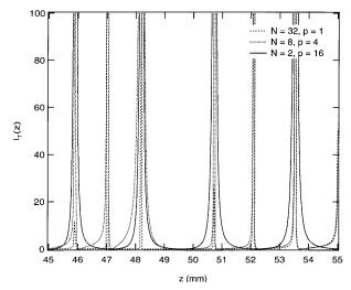
Fig. 4. Transition term  $I_T(z)$ , Eq. (15), as the diffractive element tends to the refractive limit. The same design parameters of Fig. 3 are adopted. In the purely refractive case, the transition coefficient is identically equal to one. As seen here, the basic dependence with the number of zones remains essentially unaltered, except for a scaling term, up to N = 2.
