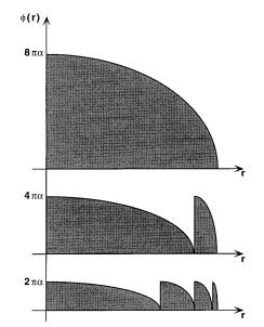
Fig. 1. Iterative process showing how the limits of a diffractive kinoform and a purely refractive lens are obtained. Only a cross section of phase function  $\phi(r)$  is illustrated. In each step the semiaperture is kept constant while maximum phase transmission  $2\pi\alpha p$  increases, where *p* is an integer. When the number of zones N = 1, we have a purely refractive lens. As *N* increases, with a subsequent decrease in *p*, the diffractive properties of the element become predominant.
