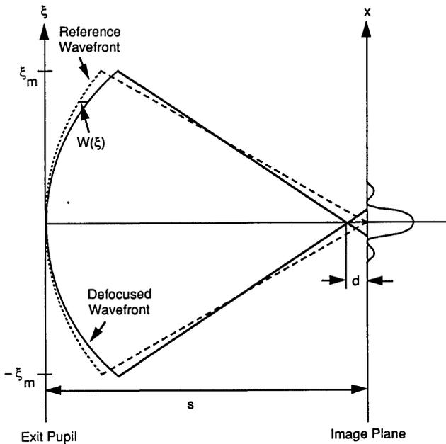
Fig. 6. Notation used for point spread function calculation:  $s$  is the distance from the exit pupil to the paraxial image plane,  $\xi_m$  is the halfwidth of the exit pupil, and  $d$  is the defocus amount.  $W(\xi)$  is the difference between the reference circle and the aberrated wavefront.
