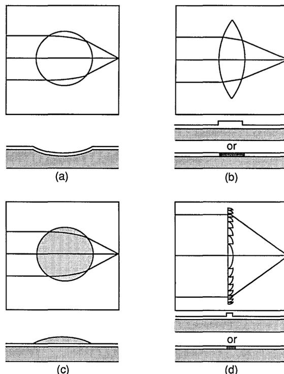
Fig. 1. Top and side views of standard types of waveguide lens: (a) geodesic, (b) mode index, (c) Luneburg, and (d) diffractive.
