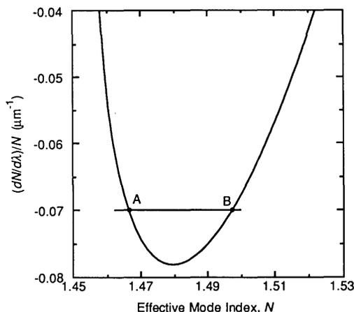
Fig. 3. Relative index dispersion of the TE<sub>0</sub> mode as a function of the effective mode index for a step-index Corning 7059 waveguide on an oxidized silicon substrate. The design wavelength is 0.6328  $\mu\text{m}$ . Each point on the curve corresponds to a different waveguide thickness. Points A and B are an example of a pair of indices which would give an achromatic mode-index lens corresponding to waveguide thicknesses of 0.35 and 0.66  $\mu\text{m}$ , respectively.
