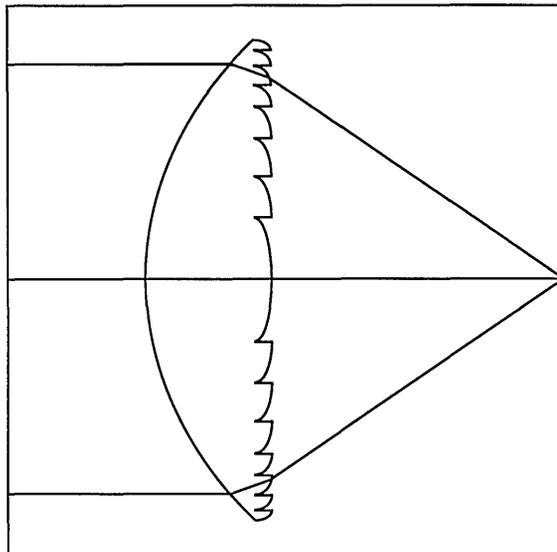
Fig. 4. Possible configuration for hybrid mode-index/diffractive achromat.
