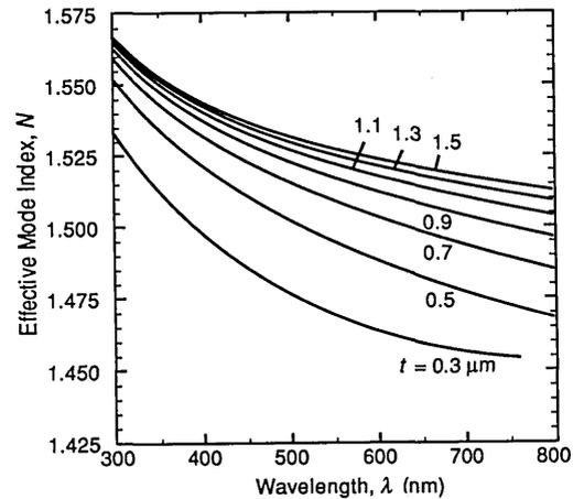
Fig. 2. Effective mode index for the TE<sub>0</sub> mode as a function of wavelength for various thicknesses *t* of a step-index Corning 7059 waveguide on an oxidized silicon substrate.
